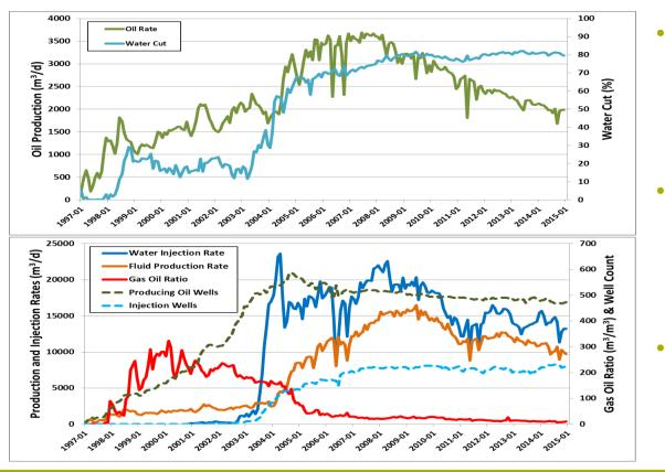
Base production is a mix of primary, waterflood, and polymer flood pads.
