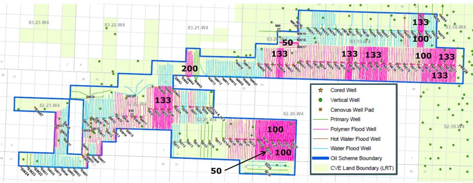
Interwell spacing distances shown are from producer to producer. Non infilled areas are at 400m spacing
