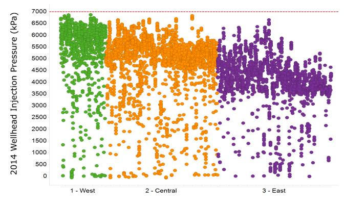
Allowable Maximum Wellhead Injection Pressure = 7,000kPa
