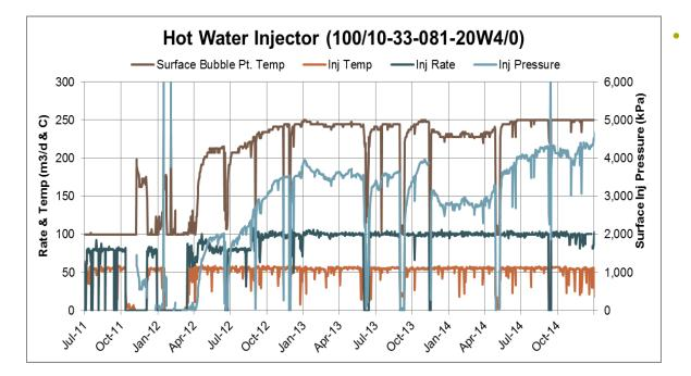
Existing primary well on pad converted to injector – casing spec not suitable for high temperature injection (~55 C max)
