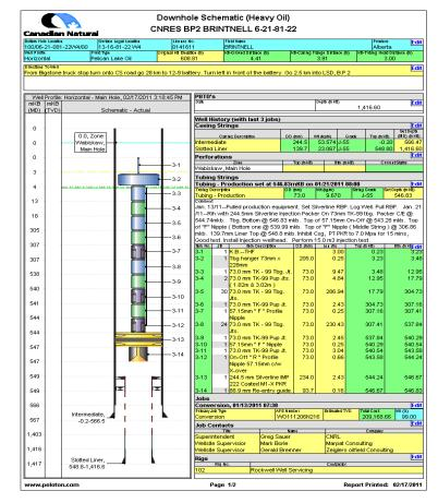
• Intermediate Casing landed in Wabiskaw sand (producers and injectors).
