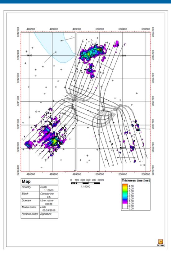
Time delay anomalies are the difference between the Devonian surface on the 2006 baseline seismic survey and the 2015 monitor seismic surveys over drainage areas A to the north, C to the west and D to the east.
