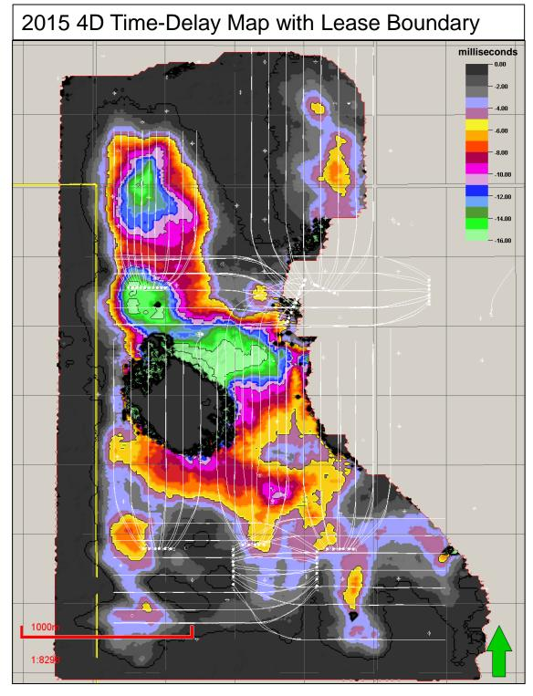
Time delay anomalies are the difference between the Devonian surface on the 2003 baseline seismic survey and the 2015 monitor seismic surveys.
