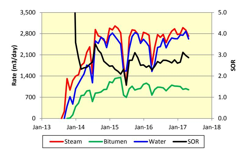
Medium Performance Pad: SAGD pay is under an associated gas cap and above bottom water. There has been no particular challenge in operating this pad to date.
