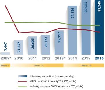
\* Phase start-up: higher steam requirements with low initial production \*\* Net GHG intensity includes the associated benefits of cogeneration
