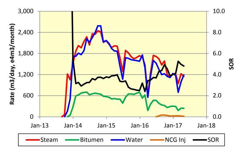
Low Performance Pad: Due primarily to injectors being drilled lower than planned making it difficult to control vapor production near heel. Well work-over to isolate the heel section of one injector resulted in better performance is expected following similar upcoming work-overs.
