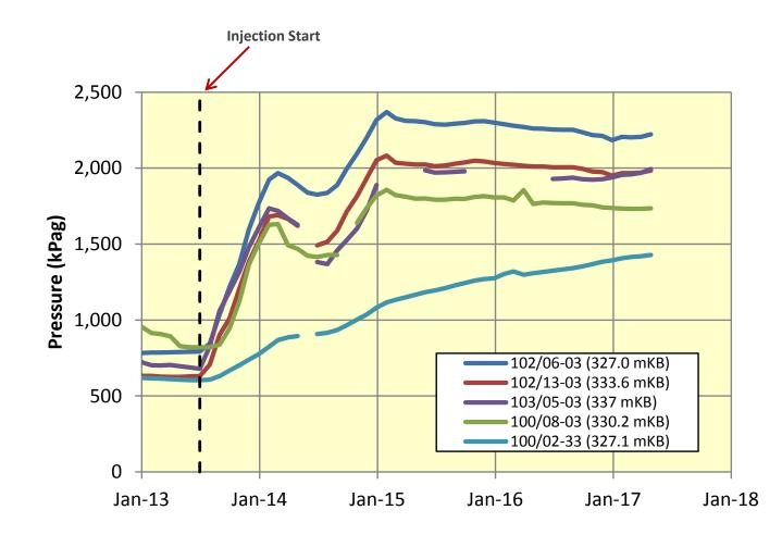
The 100/02-33 well is roughly 1,600 meters away from the active injection/SAGD area
