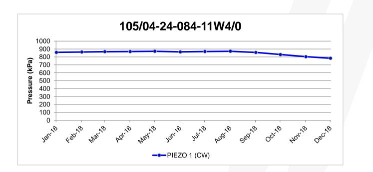
Well is deviated and has a hanging piezometer. Depth matches GR, but measures CW.
