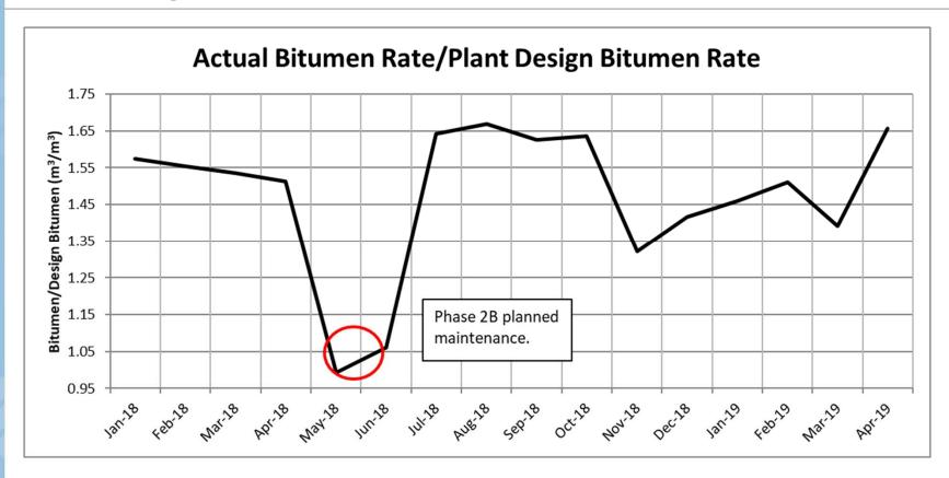
Performance over original design primarily due to operation with naphtha diluent and equipment design factors.
