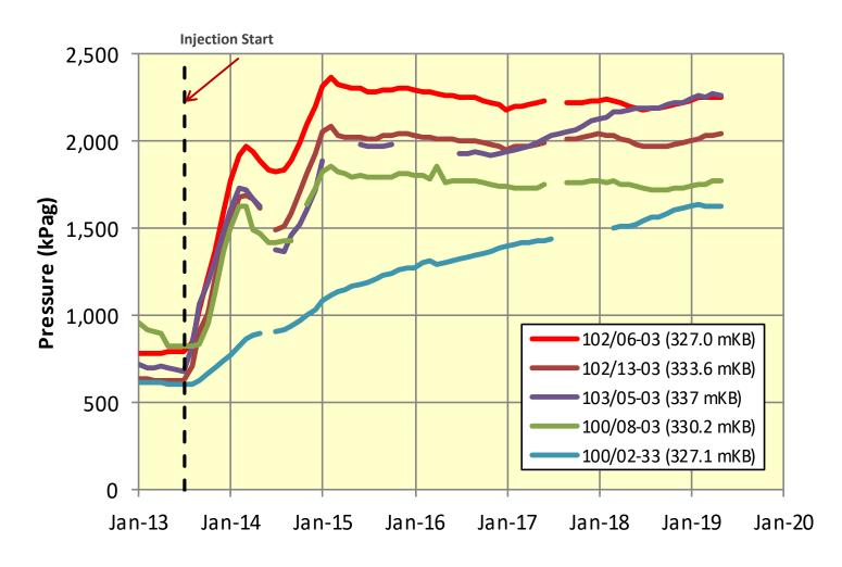
The 100/02-33 well is roughly 600 meters away from the active injection/SAGD area
