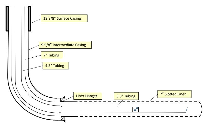
Consists of several holes placed mid-way of the long tubing to distribute steam at the middle of the well in addition to the heel and toe
