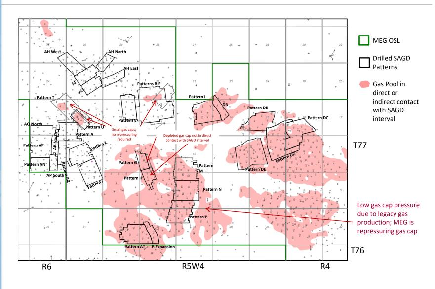
**Note**: Not all SAGD intervals in the pool wells are directly connected to associated gas
