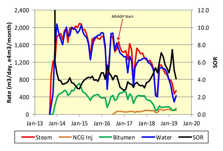
**Low Performance Pad:** Issues are suspected to be related to potential scale formation and aggravated by exposure to bottom water.
